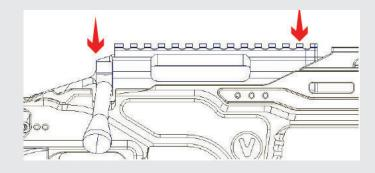
Make sure that the anti-vibration washer is on the action screws. Now engage both the front and rear action screw, but do not tighten, place the chassis on the buttpad and bounce it lightly a couple of times to make sure that the recoil lug is in the correct position. Make sure to hold the action to prevent it falling out.
