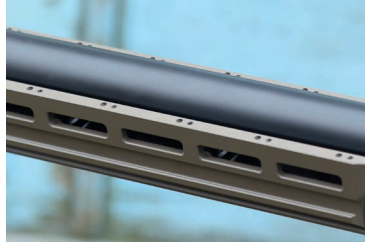
DRILLED AND TAPPED HOLES FOR MOUNTING TOP COVER AND NV BRIDGE
